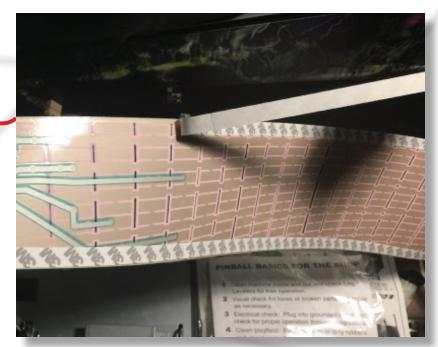
Remove the 3M adhesive tape backing from the back of the Left PowerBlade
