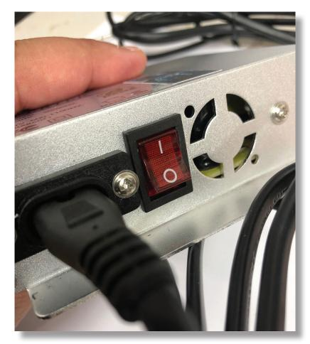
Turn the power switch to the on position.
