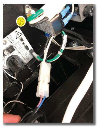
Connect the male end of the Powerblade powercord to the female connector. At this point you now have power connected.
