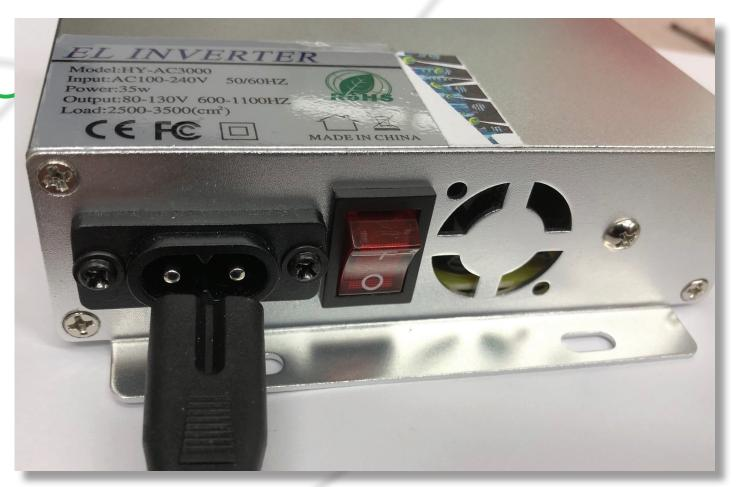
Locate the power plug for the EL converter box and plug it directly into the back side of the EL Box as shown.
