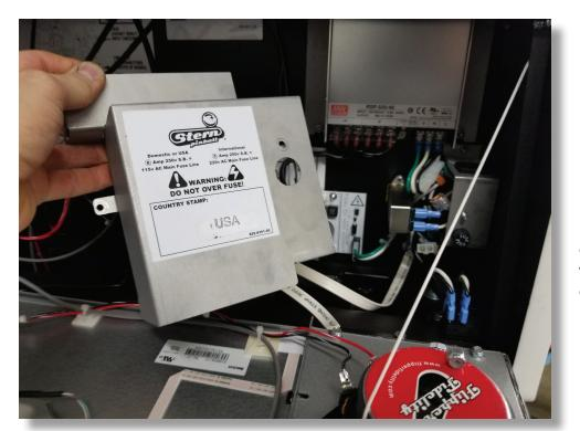
Replace the metal cover over the power area and then close up the backglass and fasten lock.
