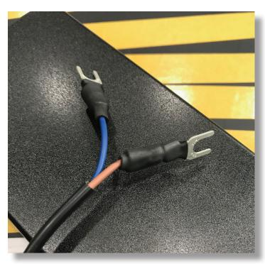
Locate the two wires coming out of the EL converter box. Note the color difference.
