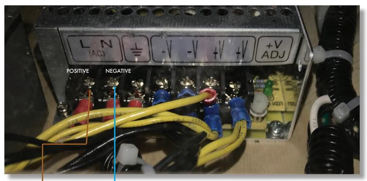
Loosen the phillips screw and connect the BROWN to the "L" Terminal Loosen the phillips screw Connect the BLUE Wire to the "N" Terminal
