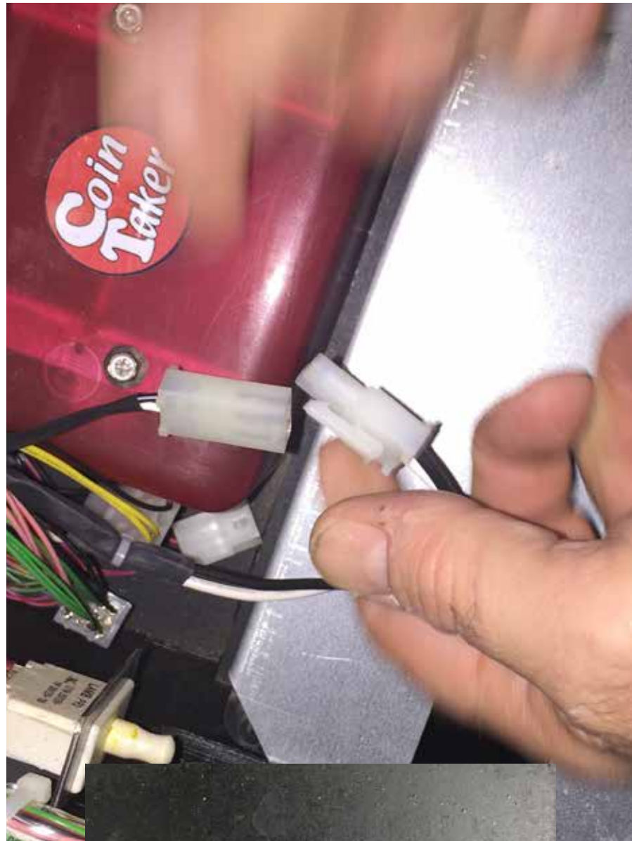
Locate the 120 Volts black and white molex wired plug and separate carefully. This plug is located on the bottom left inside the cabinet, next to the coin door.
