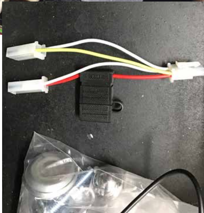
Locate the wire harness. Plug the male end of the harness into the female connector, and splice the other male connector into the female connector on the harness.
